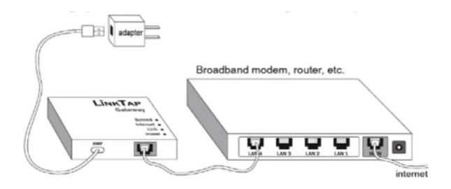
**Step 2:**Register the Gateway through LinkTap free mobile app or web app. When the registration is completed, the Synced LED on the Gateway will turn solid green.
