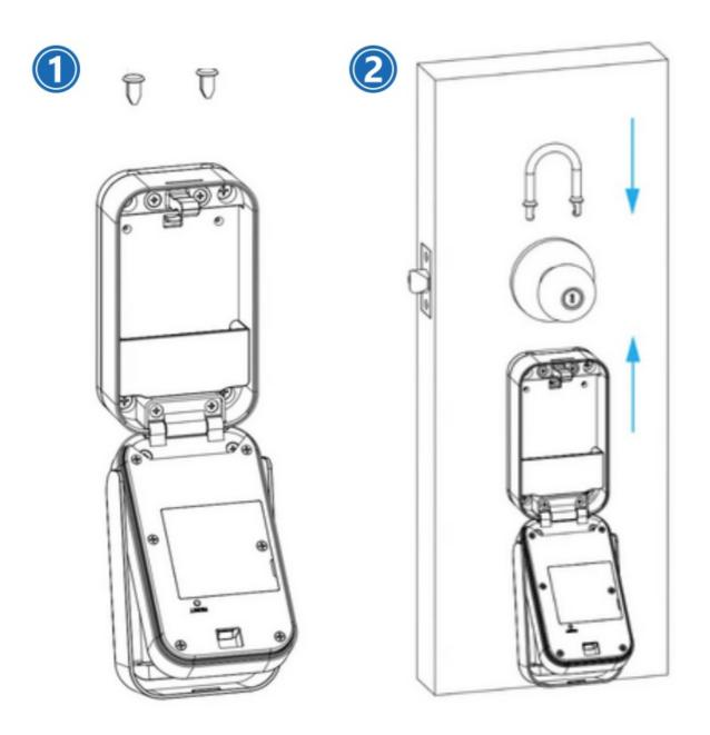
To unlock shackle, push the the Unhook button up and pull shackle out.
