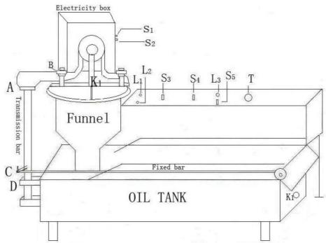
K1: To lock and hold the plunger tightly.
