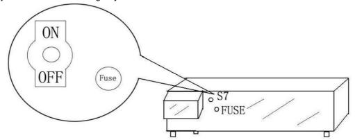
RESET: It is on the same plate as the FUSE. When the heating temperature is over 200°C, machine's power is cut. And then you screwto open it and press it to restart the machine.
