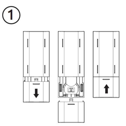
**Step A:** Locate the battery compartment on the back of the remote. Push down and away to slide the compartment cover off.
