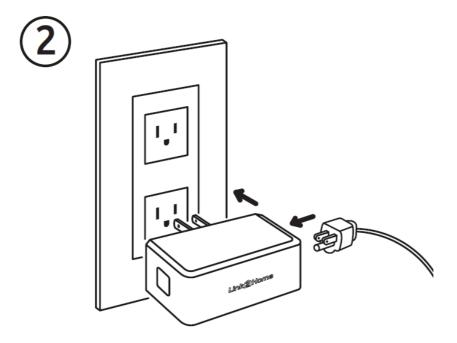
Plug the receiver into a standard AC electrical wall socket. Plug the appliance into the receiver outlet.
