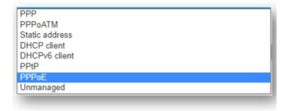
Other options include; PPP, DHCP Client, or PPPoE. I would always recommend that you bring up the default interface statically as well as upon boot. NOTE, there is options here that can render the device not reachable, and then a factory reset would be the only option.
