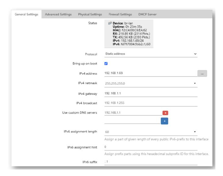
Here, you have options to select what protocol you wish, this could be used on the ethernet or any other interface. The default option is static address, where the br-lan is statically configured.
