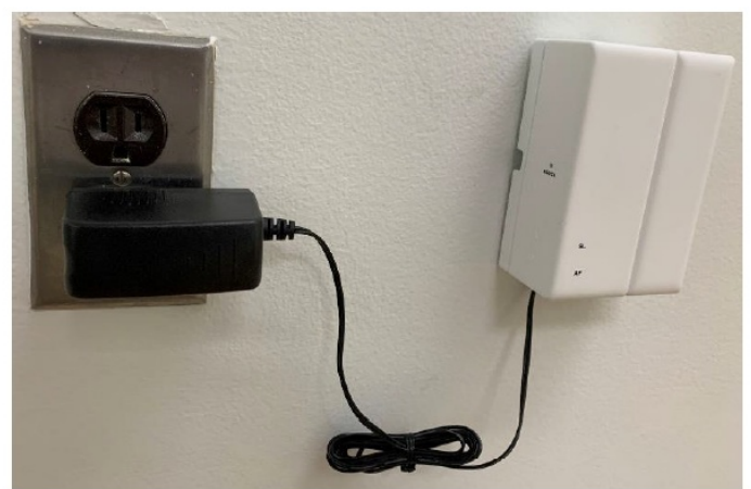
Figure 4: Side view of Access Point attached to Power Cradle AC Power
