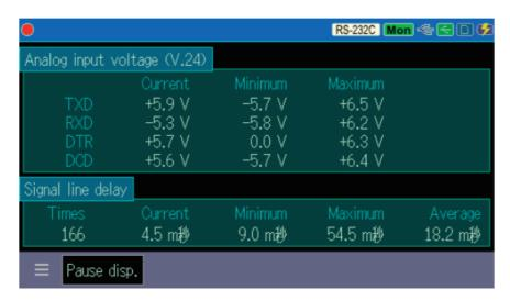
Press [RUN] to display the delay time and voltage (max./ min.).
