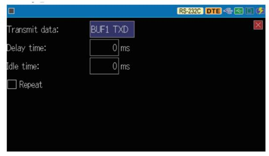
PROGRAM Mode [LE-3500XR Only] You can easily test a communication protocol that involves condition judgment using a test program created using dedicated commands.
