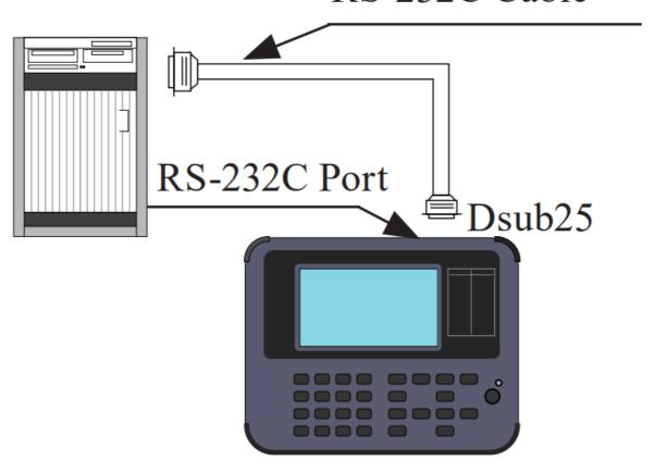
DTE device —Straight cable —Analyzer (DCE setting)
