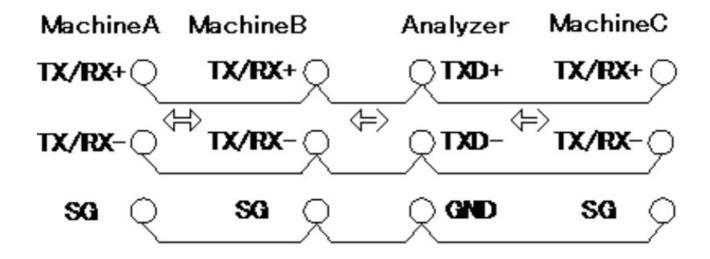
If the analyzer is located as the terminal of communication line, set the Terminal resistance 120  $\Omega$  jumper pin to be "1" on the interface sub board. (JP1: TXD, JP2: RXD)
