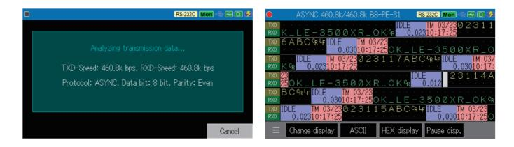
If you touch "Cancel" or press [STOP] or [ESC] before starting measurement, the communication condition analysis process will be stopped and the current communication condition settings will not be changed.
