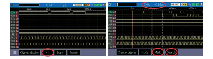
The red vertical line is the trigger point. At first, cursor C (blue dotted line) and marker M (red dotted line) overlap the trigger point.
