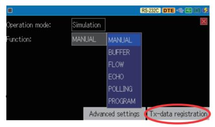
For Simulation, select DTE or DCE mode and polarity.
