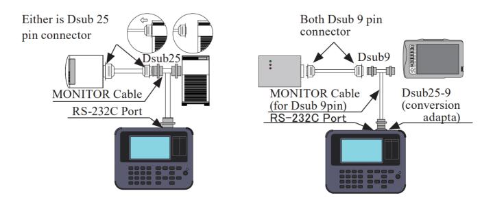
If the connector of either target device is Dsub 25 pin, use attached Dsub 25 pin monitor cable (LE25M1) to connect to the analyzer.
