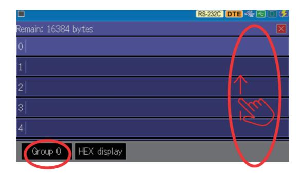
Input the data to be transmitted in HEX by [0] to [F]. Copy and paste of the data are available by [ENTER], [ $\blacktriangleright$ ], and  $\blacktriangleleft$ .
