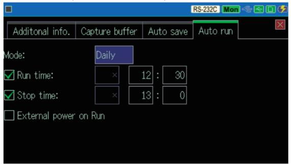
With the settings on this screen, measurement starts at 12:30 every day and ends automatically at 13:00.
