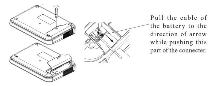
Battery is necessary for saving data in the storage (USB flash drive etc)when having the power shortage. Insert the battery all the time.
