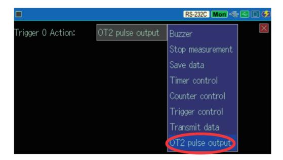
Regardless of the trigger action setting, it outputs outputs an L pulse of about 1 ms to the external trigger output terminal OT1 when any trigger factor matches.
