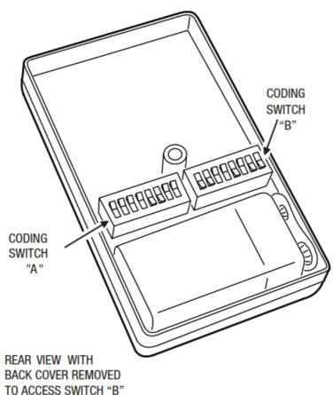
Switch "B", under the back cover is designed for use with less-frequently changed codes, such as a community gate operated by Push-button "B". The code set into Switch "B" must be identical to the code set in the receiver to be used in conjunction with Pushbutton "B".
