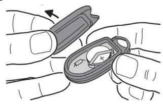
3. REMOVE THE TWO BATTERIES
