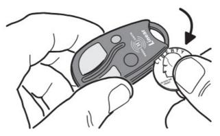
2. Remove the back of the case
