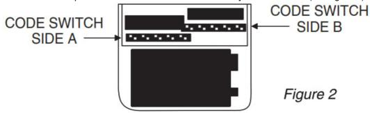
If you have a MULTI-CODE™ 3021 or 3028 two-channel receiver: Set the receiver and transmitter (side A and B) code switch positions 1-9 to match. The 10th position on your transmitter code switches is used for channel selection.
