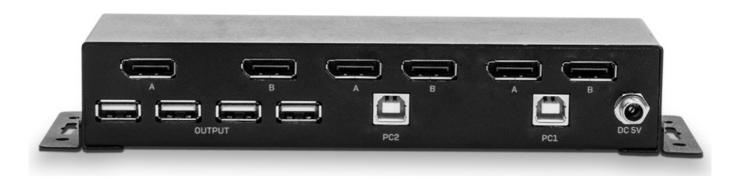
The rear panel is split into three sections. Output, PC2 & PC1 as you look from left to right. USB Input and Storage devices can be connected to the Output USB Type A (Female) Ports, Output displays connected the Output "A" & "B" Ports.
