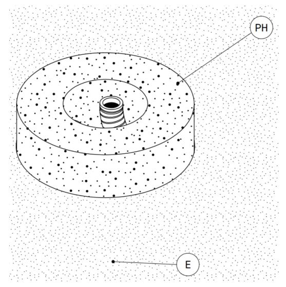
3. After the screed (E) has hardened, remove the placeholder (PH) from the screed, insert the conduits/cables (L) either on the side, or from below into the housing (4) and place the housing (4) in the cutout. Level the housing (4) flush with the floor and anchor it in the screed (E) using the grub screws (3).
