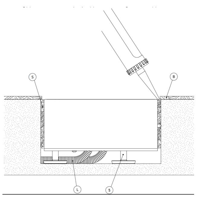
5. Finally cut the floor covering to a suitable size with a diameter of 110 mm and glue it onto the lid (1) with a construction adhesive (eg "beko ALLCON 10").
