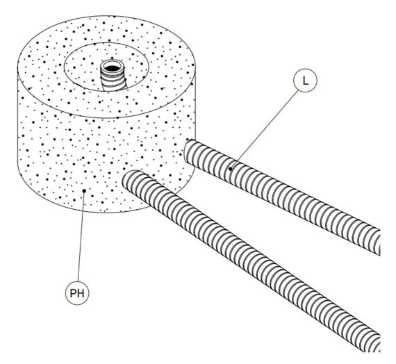
2. Now pour the placeholder (PH) with screed (E). The later construction height must be taken into account. Let the screed (E) harden.
