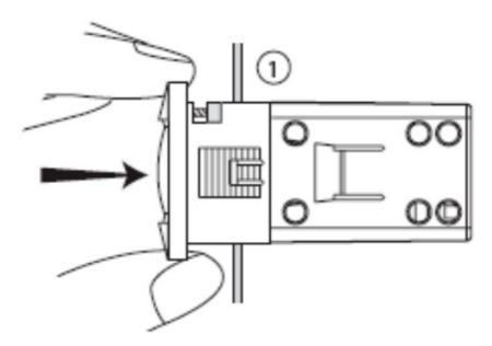
2. Slide the bracket to fix the device (step two)
