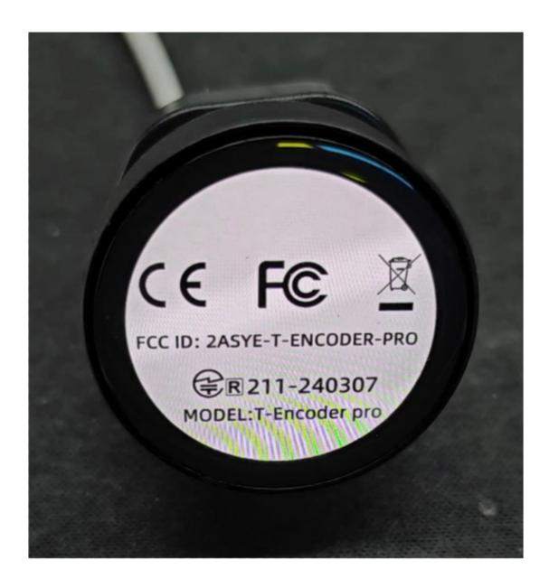
After connecting USB to power on. The screen can directly display the electronic label for 3 seconds.
