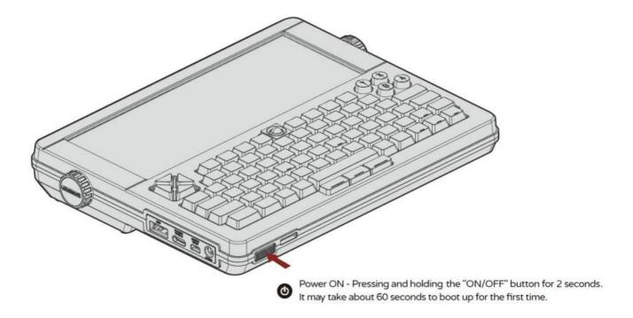
Make sure that the batteries are fully charged and installed correctly. The DevTerm can be powered by 5V-2A USB-C power supply. MicroSD must be inserted before power on. Pressing and holding the "ON/OFF" button for 2 seconds. For the first time of booting up, it will take about 60 sec.
