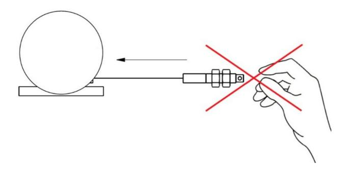
Always keep the wire aligned not to damage the equipment (maximum deviation: 3°).
