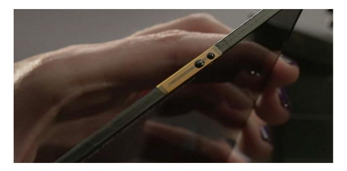
Using small RFID sticker tags, the FRS-Light detects the type and position of each inserted filter and displays the information so that the cam op and AC can easily keep track of what is in the matte box.
