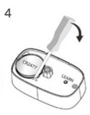
• To insert the battery, gently tilt at an angle towards the metal contact at the edge of the battery slot. Ensuring the positive symbol (+) is facing upwards, with very light pressure, push the battery down (5).
