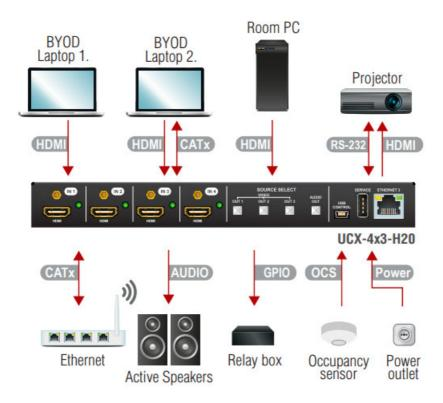
**HDMI** Connect an HDMI source (e.g. BYOD laptop or room PC) to the HDMI input port.
