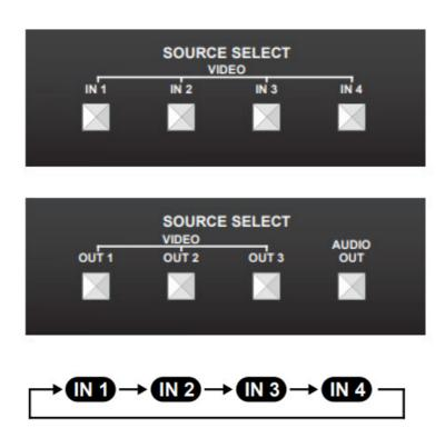
Use the **AUDIO OUT** button for switching the audio source to the analog audio output. The sequence is the same as above.
