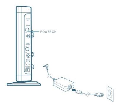
1. Redcat Access should be placed within 7 feet of an electrical outlet and on a surface about 4-6 feet off the ground.
