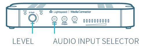
Adjust the volume as needed by pressing the Audio Input selector and adjusting the level knob as needed.
