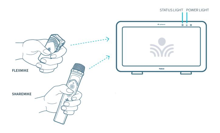
If the microphone is out of range, it will automatically shut off after 30 minutes of trying to reconnect. Once you are back in the classroom, or in range, simply press and hold the power button on the microphone to power it up.
