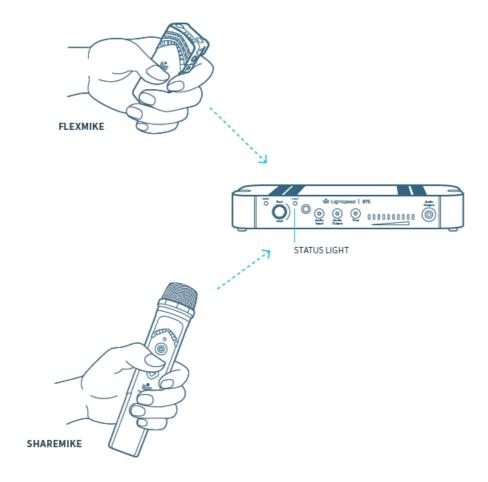
If the microphone is out of range, it will automatically shut off after 30 minutes of trying to reconnect. Once you are back in the classroom, or in range, simply press and hold the power button on the microphone to power it up.
