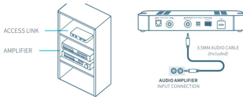
1. The Access Link box is typically located near the classroom audio amplifier.
