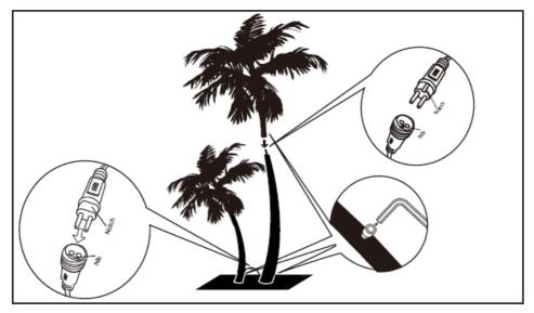
4. Connect the power adapter. Fix the base with ground stakes (when using outdoors).
