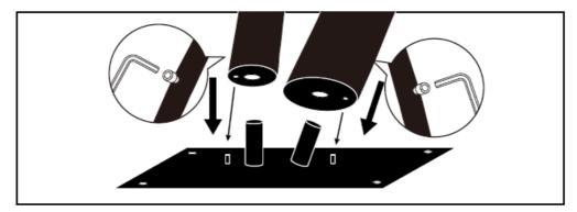
3. Find the wire joints inside the upper & bottom trunks. Connect the joints, insert the upper trunk into the bottom one and fix with screw.
