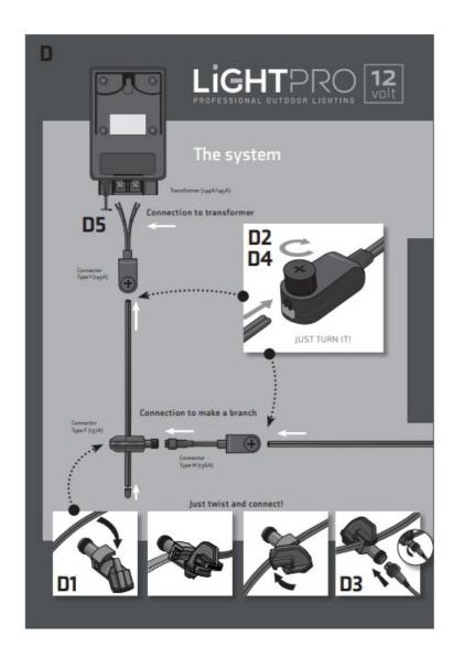
The Lightpro cable system consists of a 12 volt cable (50, 100 or 200 metres) and connectors. When connecting
