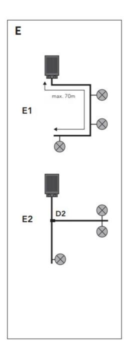
Lay the main cable through the entire garden. When laying the cable, keep the (planned) paving in mind, ensure that later on lighting can be fitted in any position. If possible, apply a thin PVC tube under the paving, where, later on, a cable can be led through.
