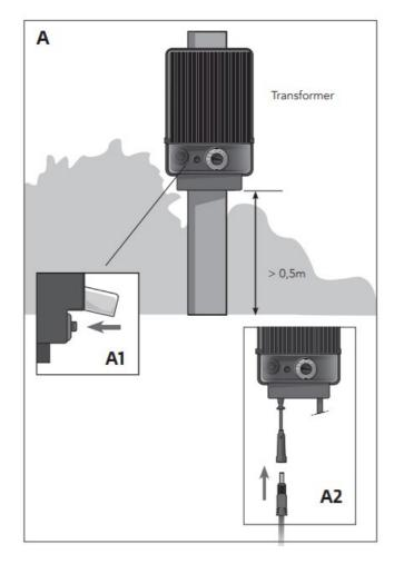
Mount the transformer with the setting knob pointing downwards <Fig. A>. Attach the transformer to a wall, partition or pole (at least 50 cm above the floor). The transformer is equipped with a light sensor and a time switch.
