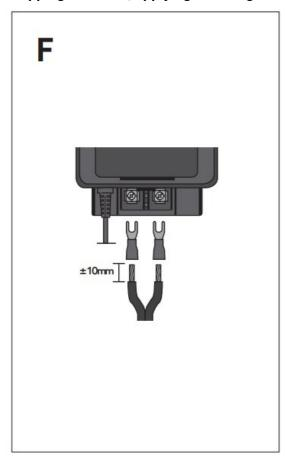
Another possibility to connect the 12 volt cable to the transformer is the use of cable lugs. Strip about 10 mm of insulation off the cable and apply cable lugs to the cable. Push the cable lugs under the connections on the transformer. Firmly tighten the screws and make sure that there is no insulation between the connections **Fig.**
