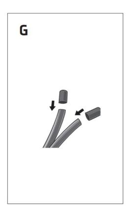
Fit caps (covers) onto the end of the cable. Split the main cable at the end and fit the caps <Fig. G>.
