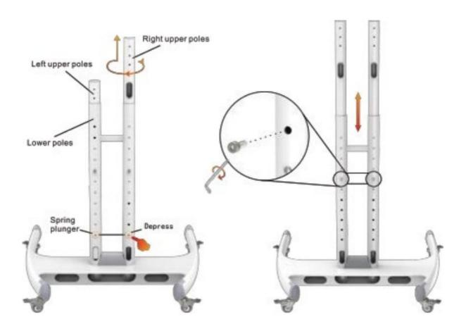
• b) And then lock it with M8\* 25mm hexagon socket screws
