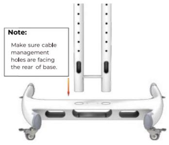
• b) Then Lock The M8\*25mm Inner Hexagonal Screws On The Bottom And Middle Of The Round Tube.
