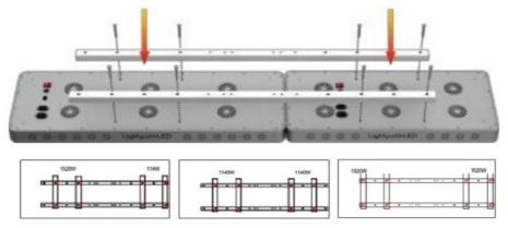
Step 7A: Install The L-Shaped Bars
