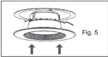
5. Ensure the three retention springs of the LED Retrofit Downlight (A) are rotated in the proper position for maximum hold in the rough-in section. Center the Downlight in the housing opening. Avoid interference with anything protrudingfrom the rough-in section walls. Push it straight up until it is tight against the ceiling (Figure 5).
