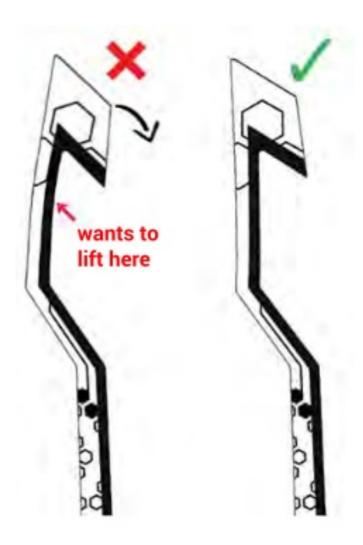
Try to avoid repeatedly unpeeling the LED strips to reposition. They may not be as sticky after multiple attempts. You also run a small risk of accidentally breaking the circuit inside the LED strip.
