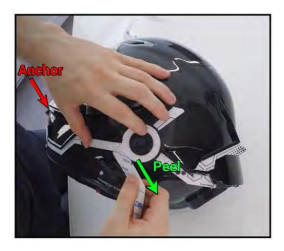
**TIP**The LED strips naturally want to follow a straight path. If you try to bend a strip laterally, while laying it down, the edge will tend to lift. Try to avoid this IF possible.
