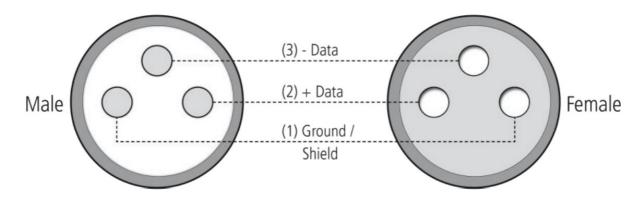
Resistance 120 ohm // 1/4 w between pin 2 (DMX-) and pin 3 (DMX+) oft he last fixture.
