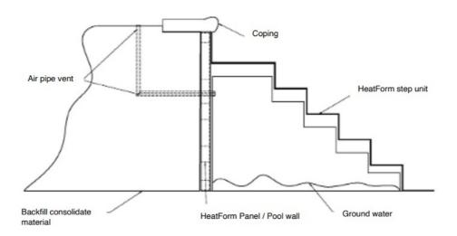
**Please note:** If there is any chance of ground water ingress into the pool shell it is recommended to install a vent kit through the wall. This is to allow any trapped air to be released and avoid any damage to the pool lining. See the example illustration of the vent system installation.
