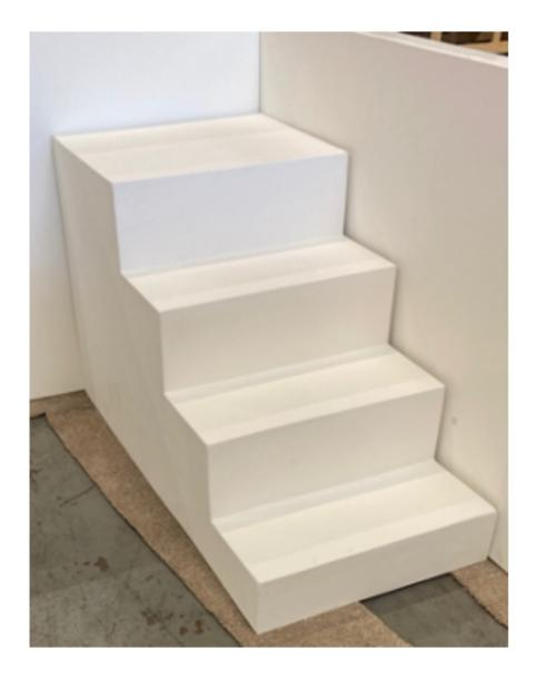
Place the step unit flush with two edges of the pool wall in the corner that you wish to have access to the pool. Bead the wall edges of the step with the supplied CT1 to seal the gap between the edge of the step and the wall. The HeatForm steps are simply installed on the floor of the pool shell prior to installing the pool liner.
