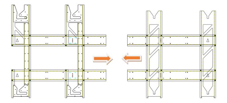
Insert the beam reinforce plate(item 5) to fixing the screw hole position.
