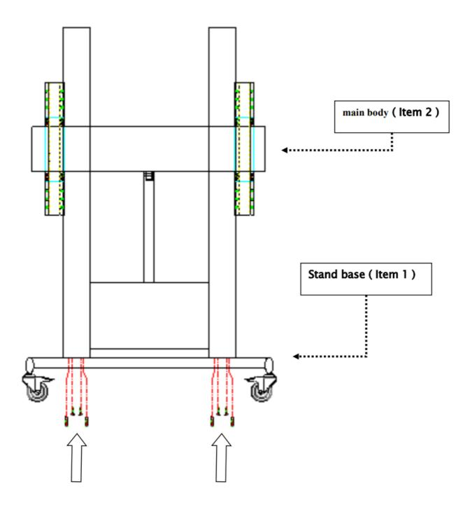
Use 8pcs M8X40 hexagon socket head cap screws (item 7) to install the stand base .
