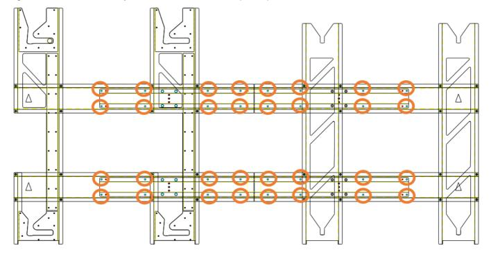
Step3. Install the panel mounting plate to the main body.
