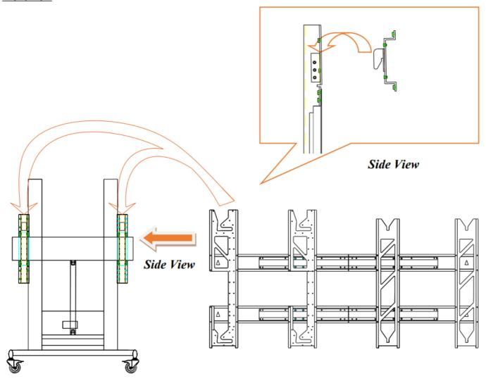
Hang the assembled back frame to the corresponding buckle points of the stand.
