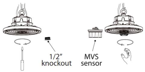
3b Mount the High Bay Low Voltage MVS Controller with Bracket (RAAS):
