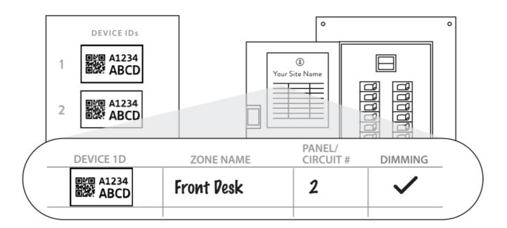
For setup and maintenance, we provide two Lightcloud Device Tables with the Gateway: one that you can attach to your panel and one to hand off to a building manager. Attach the Device Identification stickers included witheach device to a row, then write in additional information, such as Zone name, Panel/Circuit Number, and whether or not a zone uses dimming.
