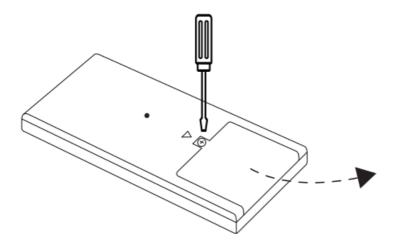
2. Install CR2032 battery in the compartment positive (+) side up
