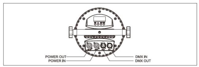
Connect the included XLR/DMX cable to the output on the DMX controller, the other end to the signal input "DMX IN", this way you can connect several devices in one chain. The cable should be a two-wire shielded cable with XLR connectors and 110Ohm impedance. When connecting devices, check the diagram below. You can attach a DMX terminator to the last device in the chain to reduce signal interference.
