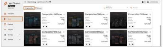
Synchronise the frame rate of animations in the settings Light Stream and Light Stream Player software. **Go to Settings->Player tab,** and in the FPS line.set the value equal to the Frame rate parameter (the window pops up when you press the left key during animation in Light Stream software).
