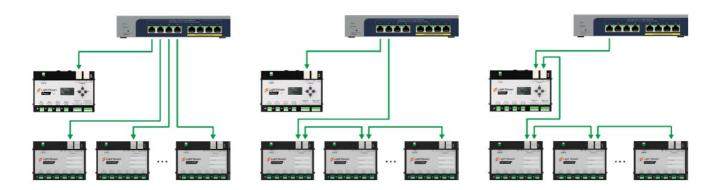
\* – If it becomes necessary to control the converters using Light Stream software, a PC with the appropriate network settings will need to be connected to the second port of the Converter, the last one in the chain. Examples of wiring diagrams can be found in the section: «Wiring diagrams» on page 4.
