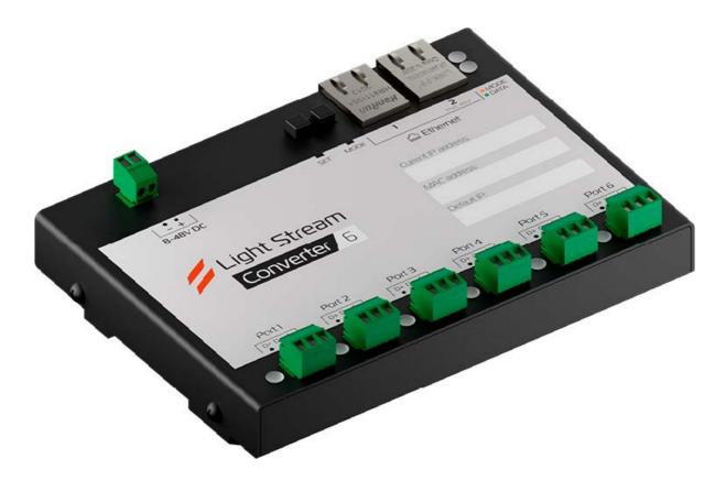
Converter with built-in Ethernet switch and 6 customisable ports. Designed for converting Art-Net signals to DMX or SPI to control lighting fixtures.
