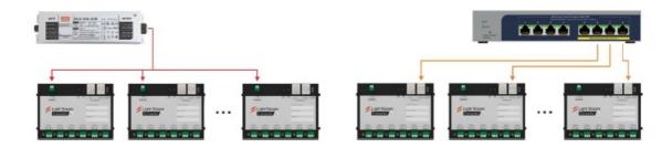
\* – in case of Light Stream Converter, only Ethernet port 2 supports PoE power supply For wiring diagrams, see: 'Wiring diagrams' on page <4>.
