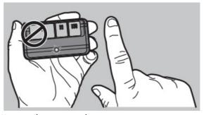
4. Press and release the Learn button on the garage door opener.
