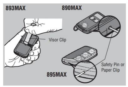
2. Press and release the remote control button you wish to use the number of times that corresponds with the garage door opener type:
