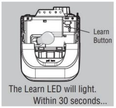
5. Press the remote control button 7 programmed in step 2 until the garage door opener lights flash or two clicks are heard.
