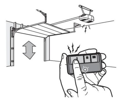
• Additional buttons on the remote control can be programmed to operate up to 3 devices such as additional garage door openers, light controls, gate operators or access control systems.
