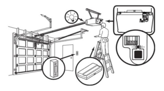
1. Press and release the "learn" button on the motor unit. The learn indicator light will glow steadily for 30 seconds.
