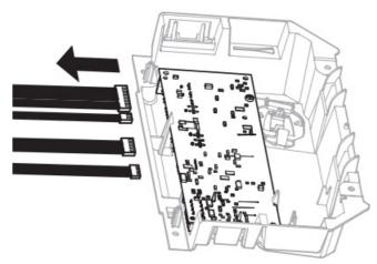
3. Remove the receiver logic board from the end panel by removing the 2 screws and releasing the 2 clips.
