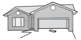
2. Press the remote control push button to close the door. The door MUST reverse when it makes contact with the board.
