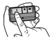
3. Release the button when the garage door opener light blinks. It has learned the code. If light bulbs are not installed, two clicks will be heard.
