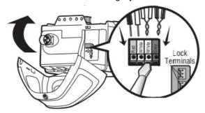
To insert or remove the wires from the terminal, push in the tab with a screwdriver tip.
