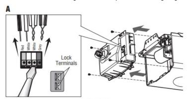
To insert or remove the wires from the terminal, push in the tab with a screwdriver tip.
