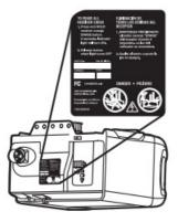
3. Disconnect electrical and battery power (if applicable) to the garage door opener.
