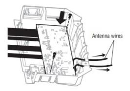
**NOTE:** Some models will require the short antenna wire to be placed in the traps of the end panel.
