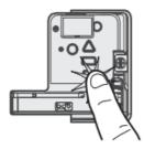
4. Press and hold the DOWN button until the door is in the desired DOWN position.
