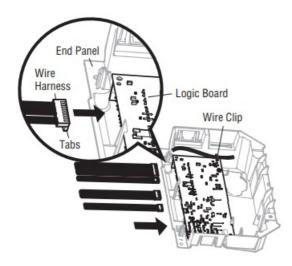
**NOTE:** If your logic board has a wire clip, use the wire clip to hold wires to the logic board.
