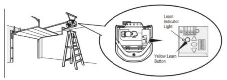
2. Within 30 seconds, press and hold the button on the remote control.
