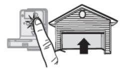
• Once the door is in the desired UP position press and release the Adjustment Button. The garage door opener lights will flash twice and the DOWN Button will begin to flash.
