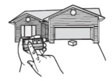
The garage door opener will not close from a remote control if the LED in either safety reversing sensor is off (alerting you to the fact that the sensor is misaligned or obstructed). If the garage door opener closes the door when the safety reversing sensor is obstructed (and the sensors are no more than 6 inches [15 cm] above the floor), call for a trained door systems technician.
