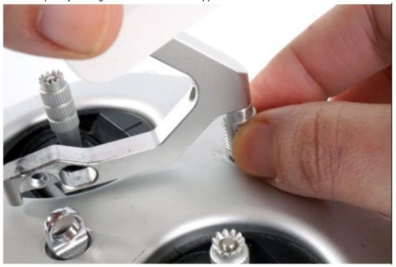
Align the LifThor Lite mounting bracket and secure lightly with the smaller screw with the smaller Hex Key (Allen key) provided.
