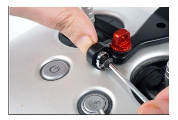
Secure the rear end of the bracket with the bigger screw and washer provided, once secured in place tighten the front screw by pushing down the bracket to align properly.
