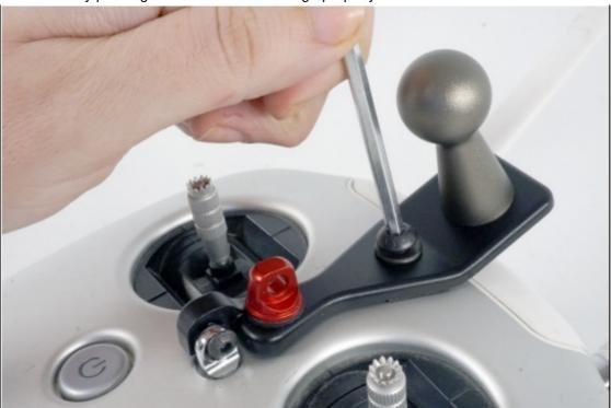
Unscrew the tightening ring from the back of the tablet clamp and place it on the ball joint.
