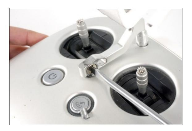
With the tips of your fingers unscrew the rear support of the bracket to remove the OEM bracket.
