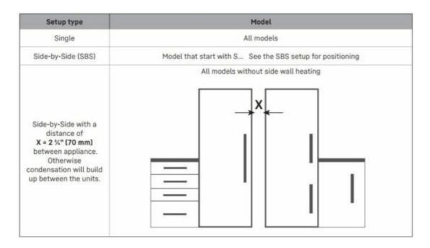
Only specific models can be combined for a side by side installations keeping always the original door opening, as they include a heating blanket in the opposite side of the handle to avoid condensation when attached together:
