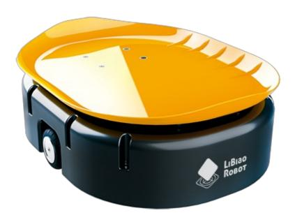
LBCRB20 Crossbelt robots are mainly used for sorting in industries of express delivery services and warehousing logistics. Operated on special sorting platforms, these robots can receive and execute orders from servers to unload parcels and transport them to designated locations.
