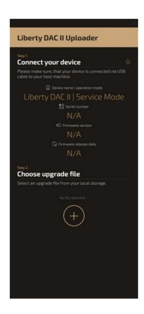
To do so, press and hold [Volume] knob button, than power-on your device by pressing and holding [Input] button (while still holding [Volume] knob button). After hearing a "click" from device, release [Input] button and than release [Volume] knob button. Your device should be discovered by Uploader App as Liberty DAC II device running Service Mode (which will be indicated by MQA diode Orange color).
