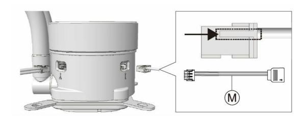
• Attention! The cable convex side on the interface shall face upward
