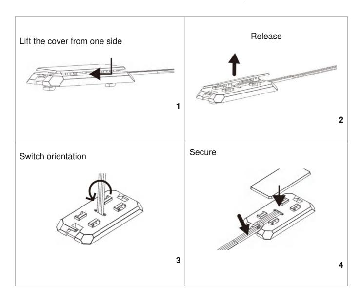
L-Wireless Receiver Installation/Installation
