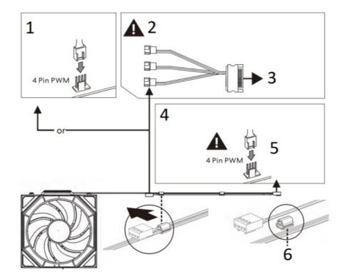
A When using the wireless receiver, each daisy-chain supports up to 4 fans
