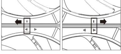
To accommodate different fan side designs, the wireless receiver allows cable output on both sides
