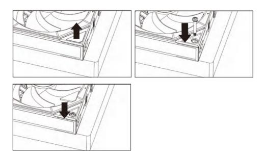
Secure the fan to the radiator and cover with the rubber pads to enhance the overall aesthetics
