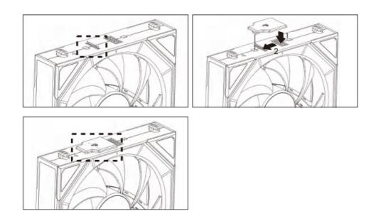
Exposed POGO PIN terminals can easily short-circuit metal components if touched accidentally. It is recommended to cover with pin cover for protection
