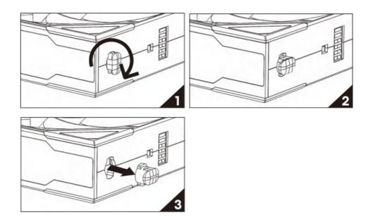
If the radiator outlet interferes with the fan interlocking key, you can remove them
