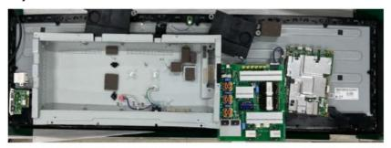
• LCD module(together with their casing) is only left after all other parts like electronic units and casing have been removed
