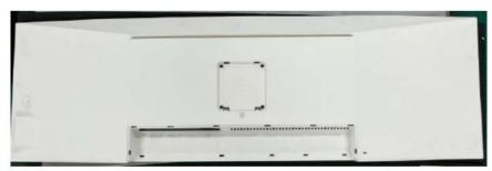
• Re-overturn the set and disaaemble screw 4EA and disassemble the PCB Monitor Only)
