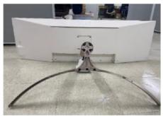
• Push button and lift the stand body and remove the screw(4EA)
