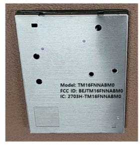
Installation of Shield-can cover
