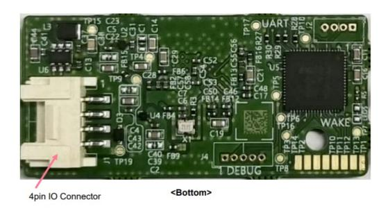
Figure 1. Radar Module Photos
